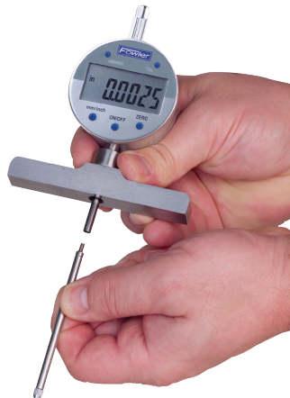
Installation of an extension rod.
