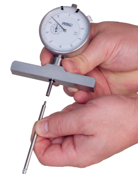
Installation of an extension rod.
