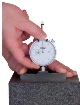
Zeroing the indicator (without the extensions) on a flat surface.
