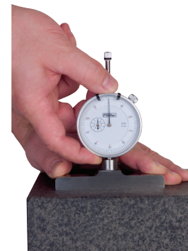
Zeroing the indicator (without the extensions) on a flat surface.
