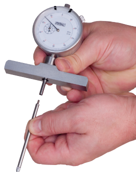
Installation of an extension rod.
