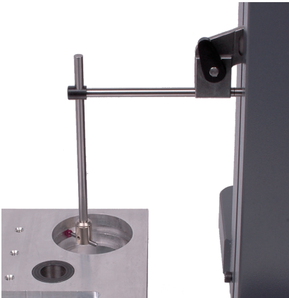
Internal groove measurements with accessories 54-199-508, 54-199-506 and 54-199-501
