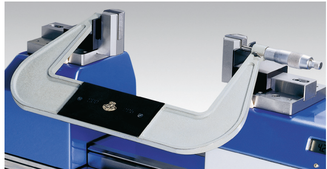
▲ Checking and setting of external micrometers from 3" to 120" (75 to 3050mm) using gage block anvils (54-190-805-0) & micrometer V-supports (54-190-825-0)
